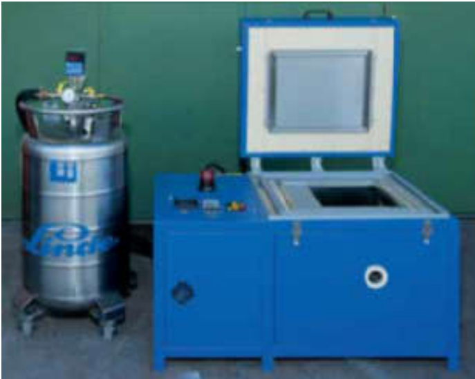
Figure 1. Set-up of cryogenic treatment in the temperature of 77 – 450 K, which consists of a well-insulated treatment chamber (right), liquid nitrogen in a Dewar vacuum flask (left), (Linde gas, sub-zero treatment of steels, technology/processes/equipment)
