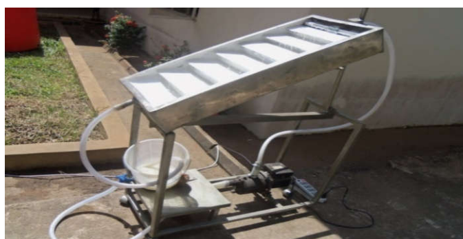
Figure 3. Side view of an inclined 6 steps fixed bed photocatalytic reactor (Source: Author)
