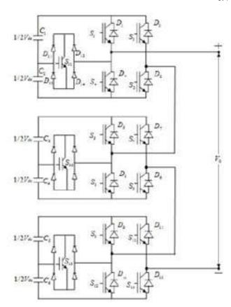
Fig. 2. Cell Configuration for Proposed Inverter
