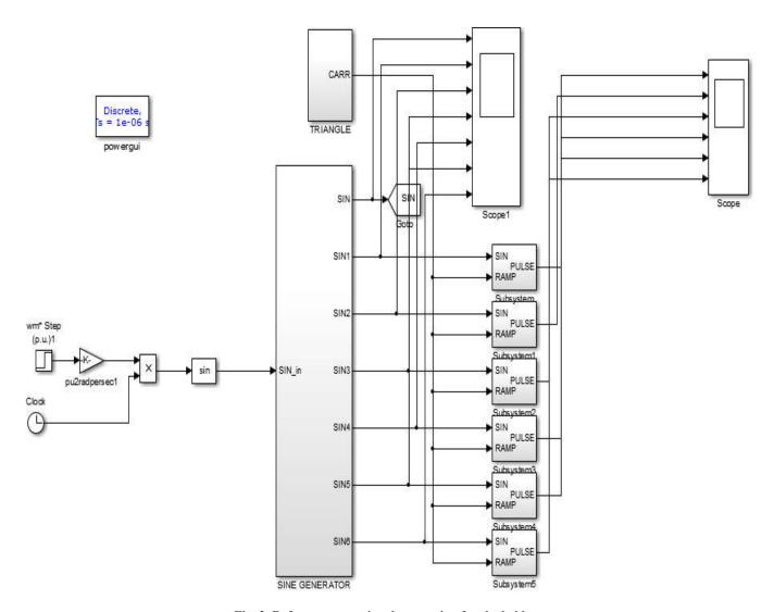
Fig. 3. Reference wave signal generation for the bridge
