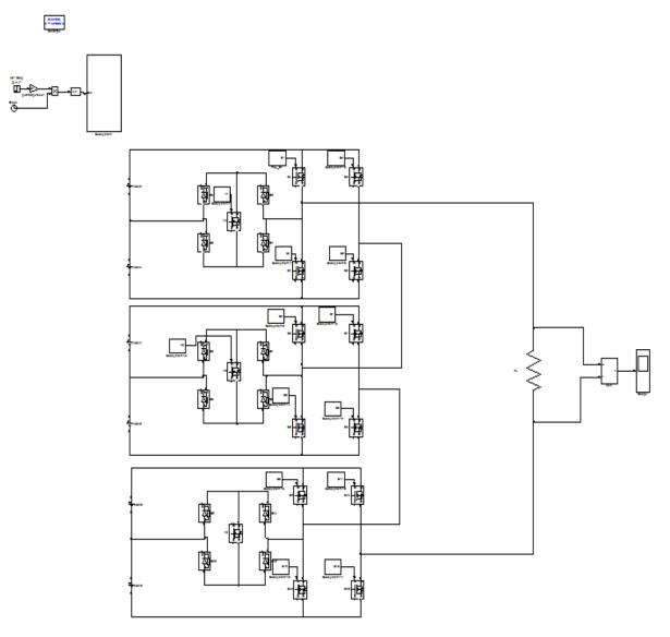
Fig.5. Matlab/Simulink for cascaded H bridge inverter
