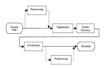
Fig. 1. Block diagram of an OCR system
