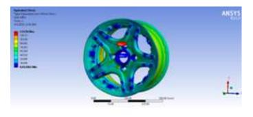
Figure 3. Static structural results on wheel
