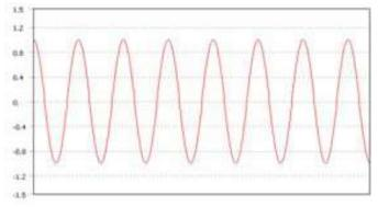
Figure 8. Constant amplitude fully reversed
