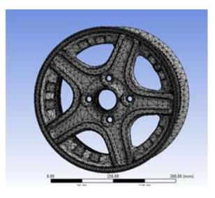
Figure 2. Meshing of Aluminium Alloy Wheel
