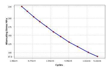
Figure 7. Alternating Stress vs Cycle
