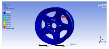
Figure 5. Fatigue life of Aluminium Alloy Wheel
